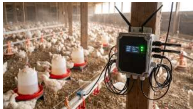
Figure 3: A sensing node installed on a support post inside a broiler house, its display reporting 26.5 °C, 68 % relative humidity and 12 ppm ammonia.
