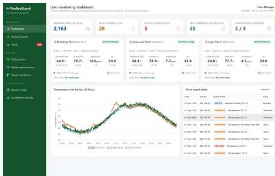
Figure 11: The monitoring dashboard, showing the current condition of each instrumented house, the alerts of the preceding day, and the temperature of all three houses over 24 hours.
